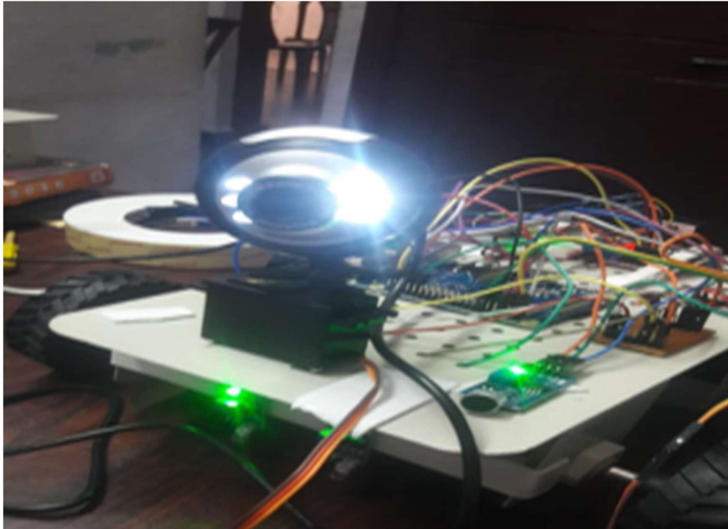
Fig. 5. The front view of the developed autonomous patrolling robot with night vision enhanced by IoT technology.
