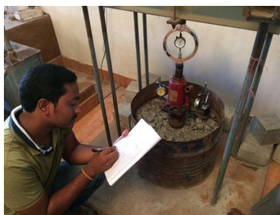
plate 5.1 Author is conducting cyclic plate load test
