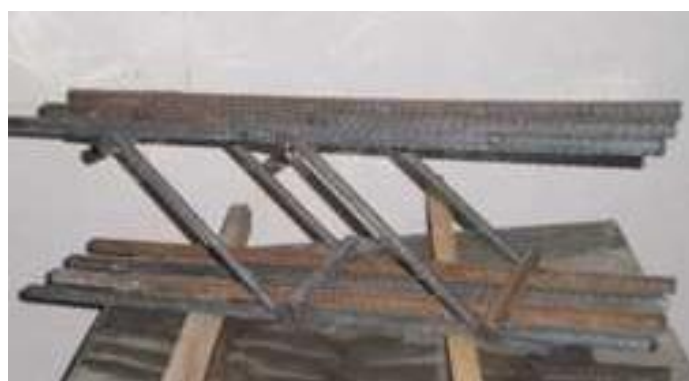
Fig. 1: Typical welded swimmer bars
