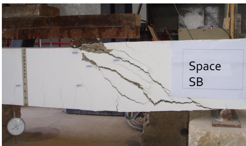
Fig. 7: Typical shear failure.
