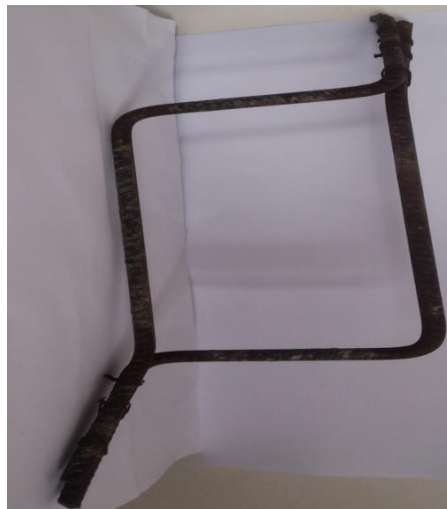
Fig. 3: Assembled space swimmer bars loop.
