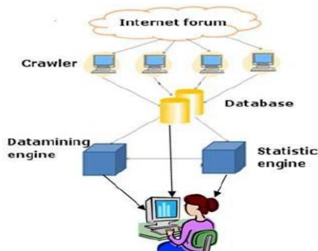
Fig – 2 System Architecture
